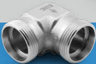
Guardian Seal Plating 0 hours Salt Spray Test
